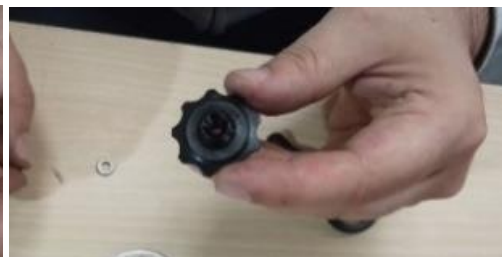
Insert the washer [9] into the pulley [18]
