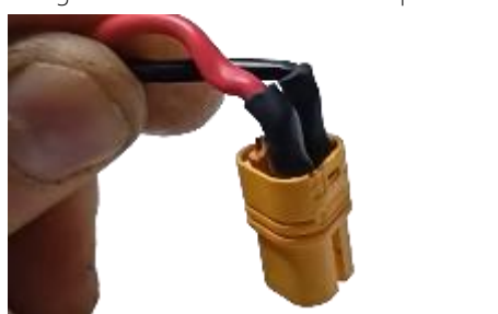
Make a fold of the cables as in the photo, it will be easier to insert the engine cover
