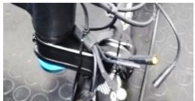
Position the splitter and secure it with a cable tie
