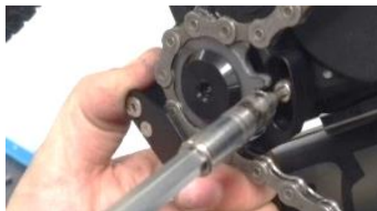
Adjust the position of the chain guide and tighten the previously fixed screw
