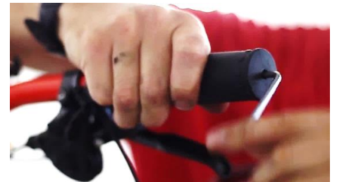
Secure the throttle with the Allen key (not included) max 4Nm
