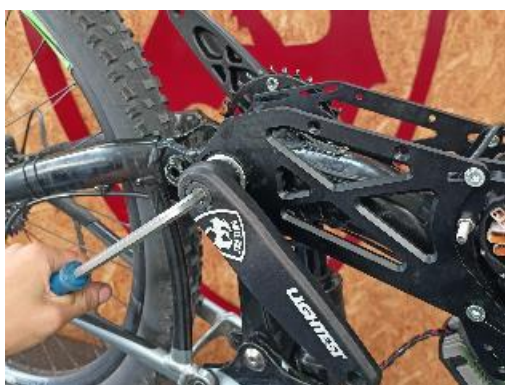
I insert all the spacers into the three holes that support the engine. Keep the nuts on the left side and the screw heads on the right.
