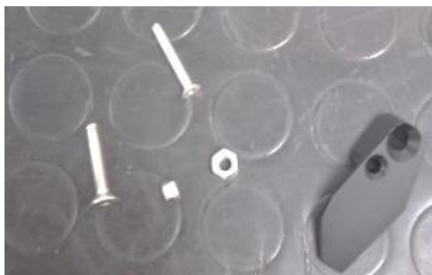
Prepare the remaining cover [19] with the M3 and M4 screws [G][H] and the relative nuts [B][C]
