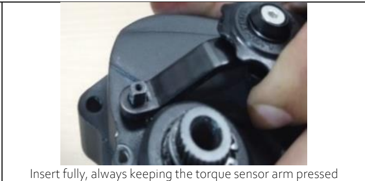
sensor assembly on the motor shaft and hold the arm down
