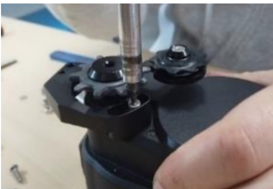
Tighten the second screw [K] lightly. Adjust the position using the buttonhole
