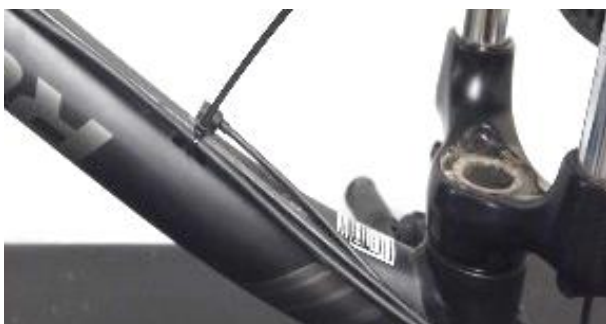
Secure the cable with a cable tie
