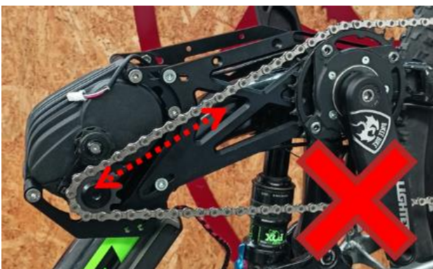
Pay attention to which chain tensioner arm you fit. The arm must push the chain to flex. If the chain remains tight the engine will not work
