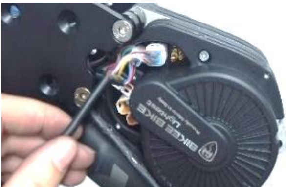
Connect the cable to the motor
