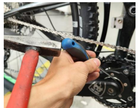
Gently tap with a hammer the screwdriver to force the ring to rotate.
