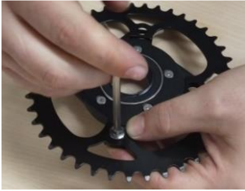
Screw the locknut with a max torque of 14Nm
