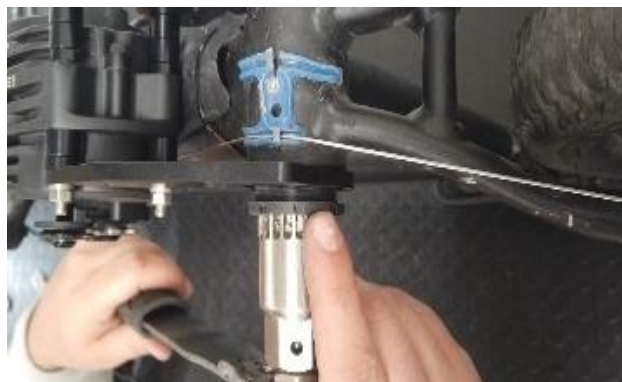
Tighten the bottom bracket
