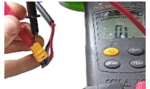
Check that the two poles just soldered are insulated and not shorted
