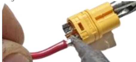
Now join the cable to the connector by heating the previously placed solder slowly and with a steady hand
