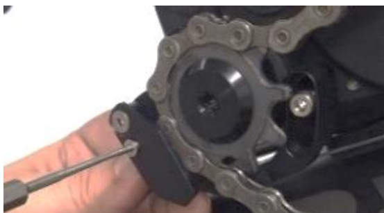
Screw as shown in the photo with the M3 screw [G] and the self-locking M3 nut [C] on the opposite side
