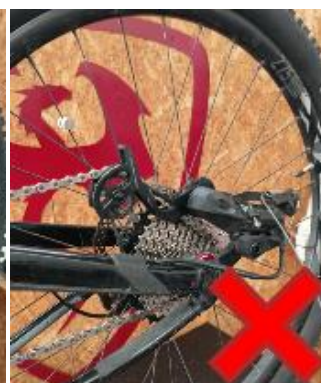
Fit the chain. You will most likely need to add some links. If the rear chain tensioner is too tight it means they need to be added. Please note that the sprocket is compatible with 11 speed or lower chain
