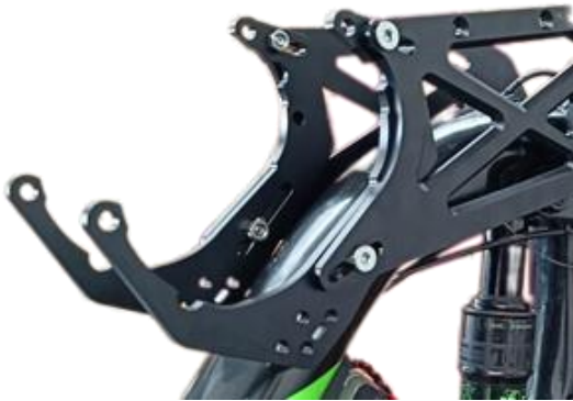
Install the two additional plates using the 4 M6x20 countersunk screws and related nuts. Don't tighten the screws too hard as we still need to adjust the tilt
