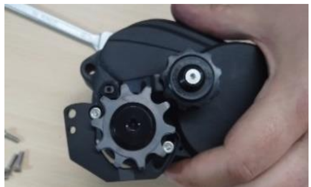
After adjustment, tighten both screws with a maximum torque of 2Nm and medium resistance thread lock
