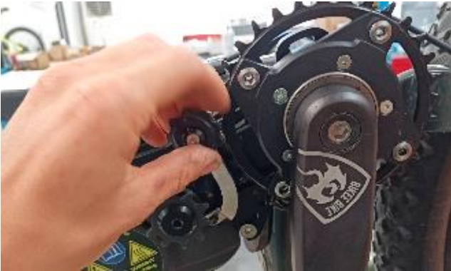
Insert the chain tensioner arm into the appropriate engine shaft.
