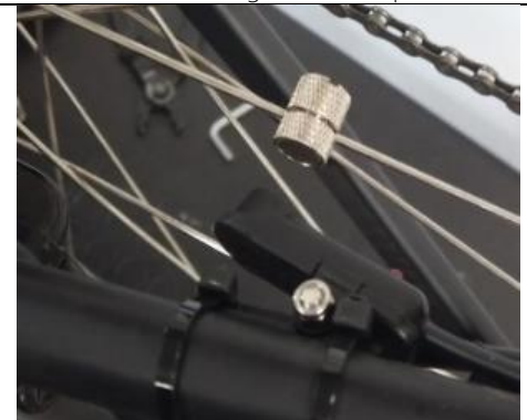
Screw the magnet to the spoke
