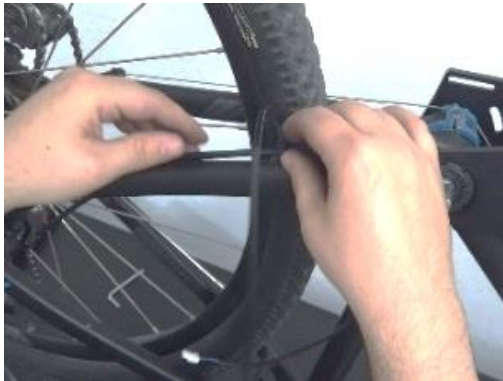
Secure the wheel sensor cable with a cable tie
