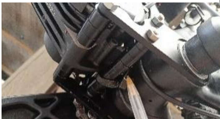
If included, add the 3rd screw with spacers for better stability
