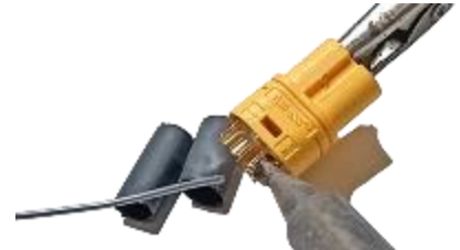
Also fill the two + and - connectors in the MT60 connector with solder
