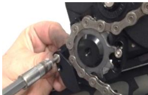
Screw as shown in the photo with the M4 screw [H] and the self-locking M4 nut [B] on the opposite side
