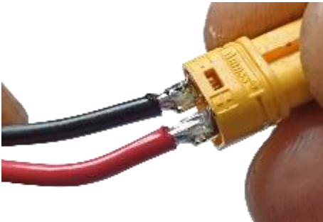
The end result must be a smooth weld. Try to pull the cable vigorously, it should not come off
