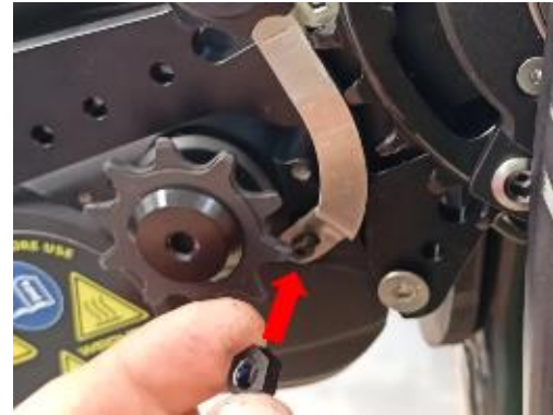
Screw the M6x0.75mm nut, make sure it is screwed straight, it is easy to insert the nut incorrectly and ruin it.
