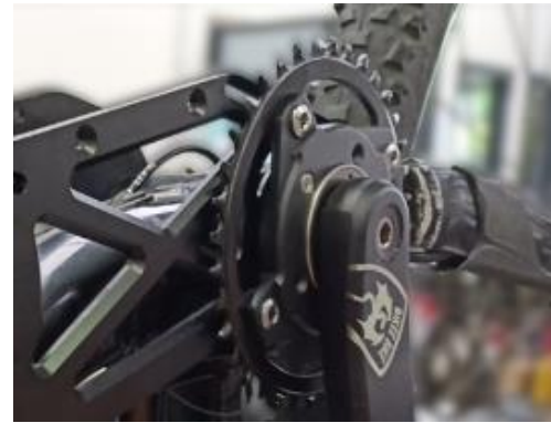
Install the crank with the entire chainring assembly assembled, tighten the screw well, bringing the crank into contact with the previously positioned spacers.
