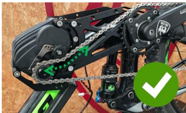
Pay attention to which chain tensioner arm you fit. The arm must push the chain to flex. If the chain remains tight the engine will not work
