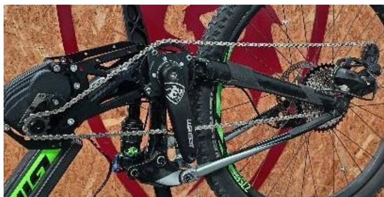
Fit the chain. You will most likely need to add some links. If the rear chain tensioner is too tight it means they need to be added. Please note that the sprocket is compatible with 11 speed or lower chain
