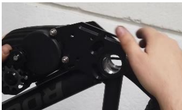
Place the motor on the bottom bracket
