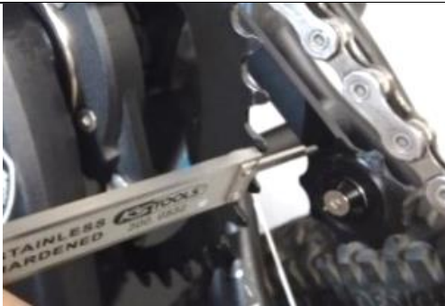
Measure the distance between the pedal chainring and the chain guide rod (in our example case it is 22.6mm)
