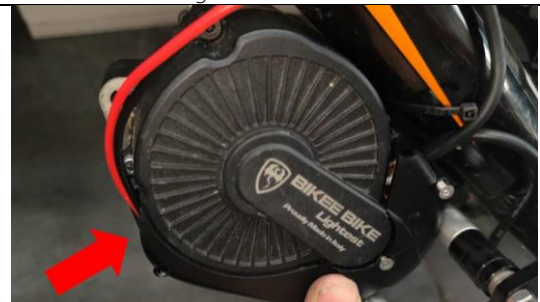
you can also use the front hole to get the cables out
