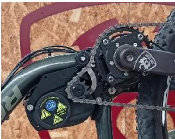
Insert the chain tensioner arm into the appropriate engine shaft.
