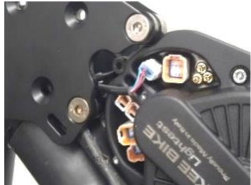
Connect the cable to the motor
