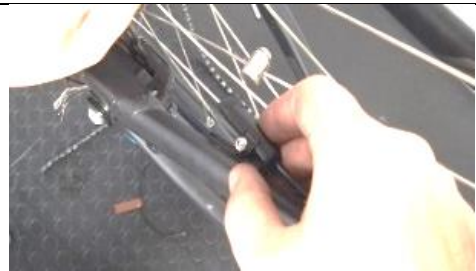
Glue the wheel sensor using the red double-sided adhesive already installed on the sensor. It is only present in some models
