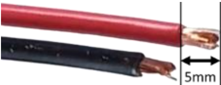
Remove the sheath for a maximum of 5mm
