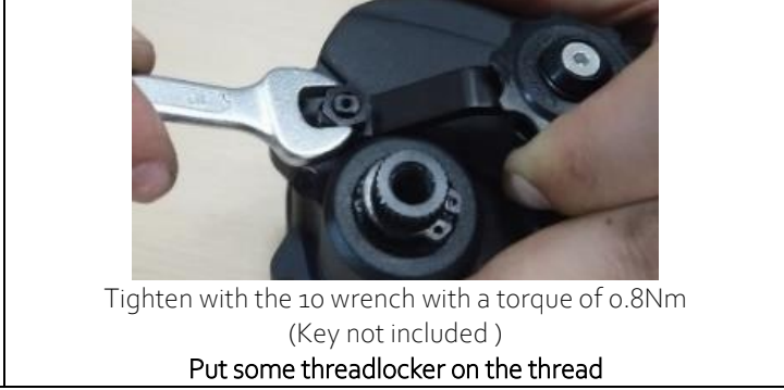
Insert fully, always keeping the torque sensor arm pressed
