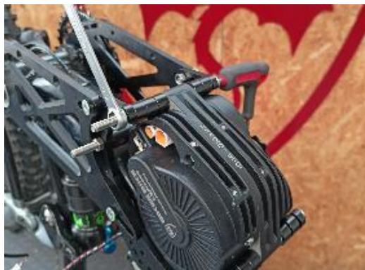
Position the engine well so that it rests well on the frame. Then tighten the three screws that support it and the 4 20mm screws. Also tighten the BSA bushings well.
