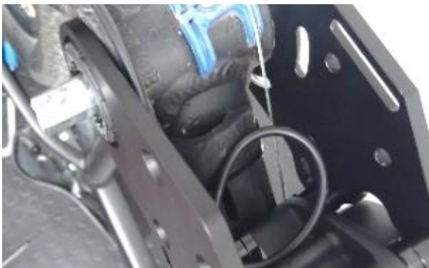
Hide the excess cable. Remember to secure the cable with cable ties to prevent it from touching moving parts
