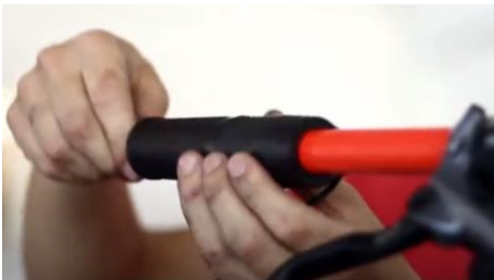
Remove the original grip, after inserting the throttle into the handlebar.
