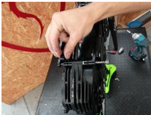
I insert all the spacers into the three holes that support the engine. Keep the nuts on the left side and the screw heads on the right.
