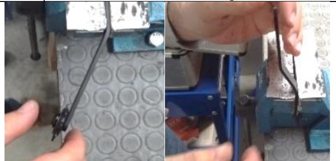
Disassemble the rod. Proceed to bend the rod to bring it to the correct distance
