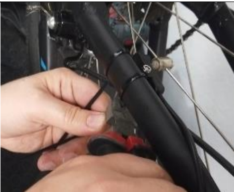
Cut off excess zip ties
