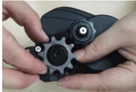
Position the larger part [20] as in the photo and screw the first screw [K] lightly
