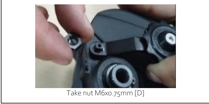
sensor assembly on the motor shaft and hold the arm down
