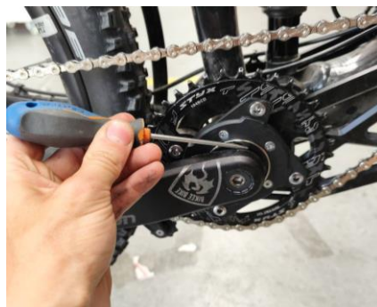
Place a flat screwdriver or similar on the hole
