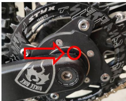
locate the hole on the freewheel ring nut
